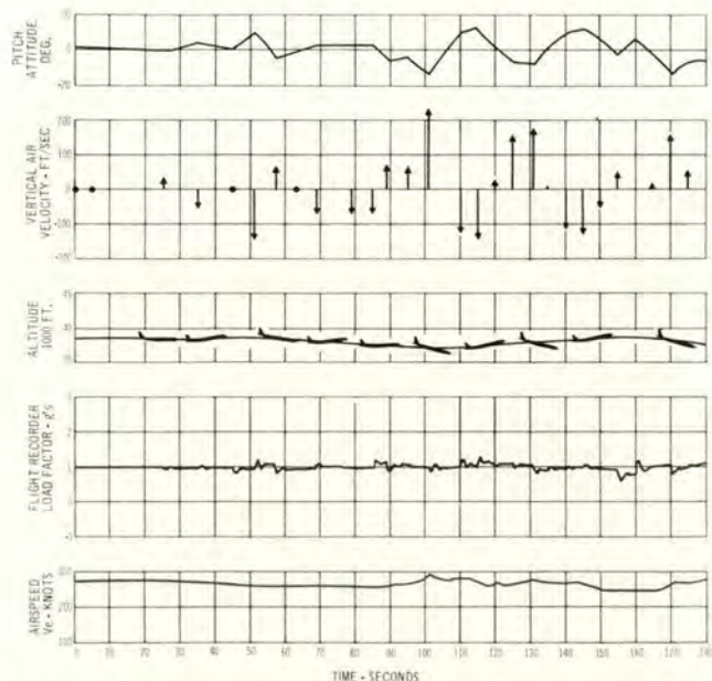
Fig 3. The indicated vertical air currents are typical of those encountered during penetration of severe turbulence. The other curves in this figure illustrate the behavior of the airplane encountering the indicated air currents without any pitch correction by the pilot.
